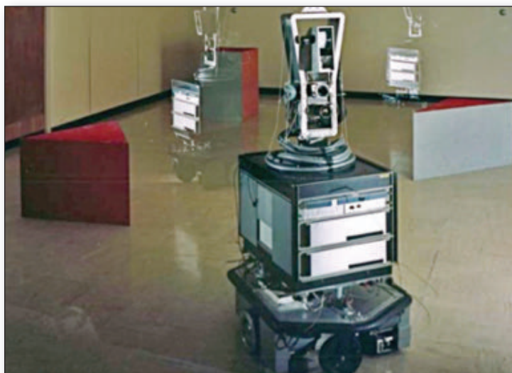
Figure 3. Triple Exposure of Shakey Moving Among Boxes.
