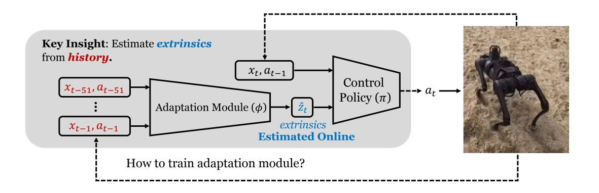
Phase 2: Train adaptation module  $\phi$  via Supervised Learning in simulation, k = 50 (0.5s) in experiments
