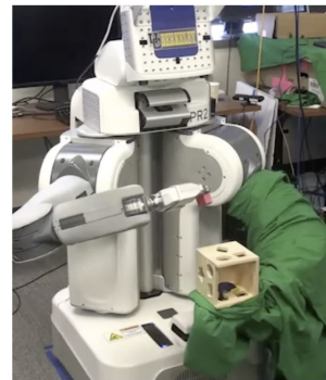
Figure 1. A PR2 learns to place a red trapezoid block into a shape-sorting cube. With Levine et al. (2016), it learns local policies for each initial position of the cube, which can be reset automatically using the robot's left arm. The local policies are distilled into a global policy that takes images as input, rather than the cube's location.
