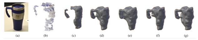
Fig. 9: Lundell et al. [139] uses drop out layers to generate 20 shape completed samples, shown in (e) - (g). The average of these samples is shown in (d) compared to [132](c). (©2019 IEEE)
