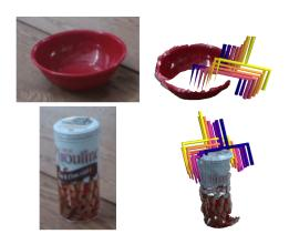
Fig. 7: An example of a grasp refinement process from [41], where the initial grasp is shown in dark blue and the final grasp pose is shown in yellow. (©2019 IEEE)
